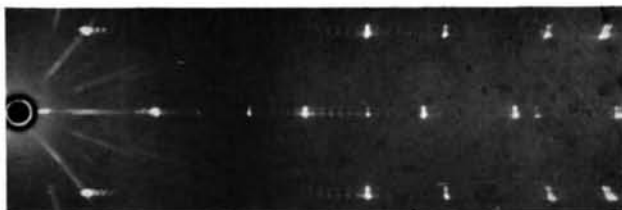
Fig. 3. a -axis 15°-oscillation photograph of the second crystal; other conditions as in Fig. 1.
